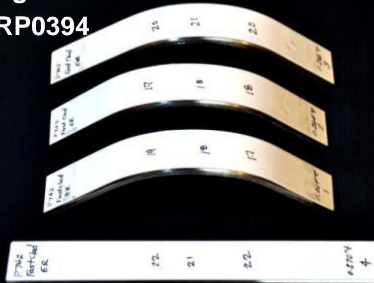
**Fast Clad ER Flexibility Test**
