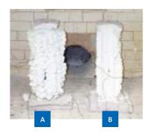
**Above:** Steel columns after fire test burn, with intumesced 'char'
