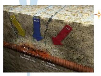
It absorbs moisture and contaminants providing an electrolyte to the corrosion cell It expands differently than steel leading to
